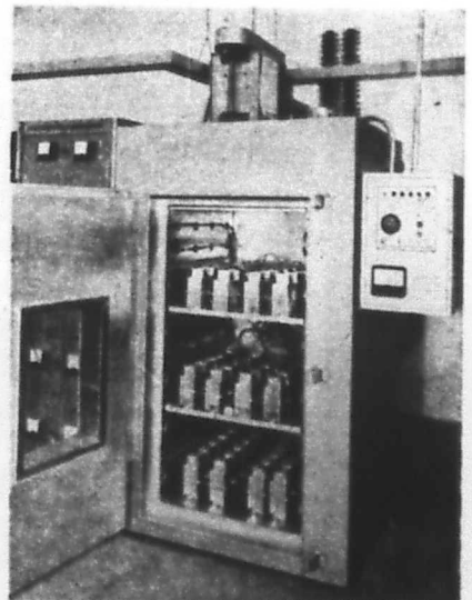
NICKEL-CADMIUM BATTERIES undergoing high-temperature life-cycle (charge/discharge) tests at new Dayton-Inland Laboratories under Air Force sponsorship to determine their reliability for space vehicle use and basic causes of battery failures.
